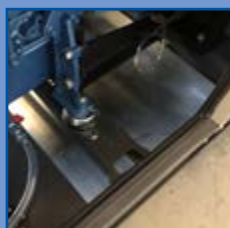
Bunded base environmental friendly - to contain the liquids in the event of a spill
